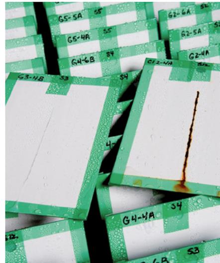
Here, aluminum and steel metal panels are continuously examined after salt spray testing and compared over a period of 500-2000 hours for any corrosive deterioration or defects on the metal surface. Advantage: Dynasylan® HYDROSIL.
