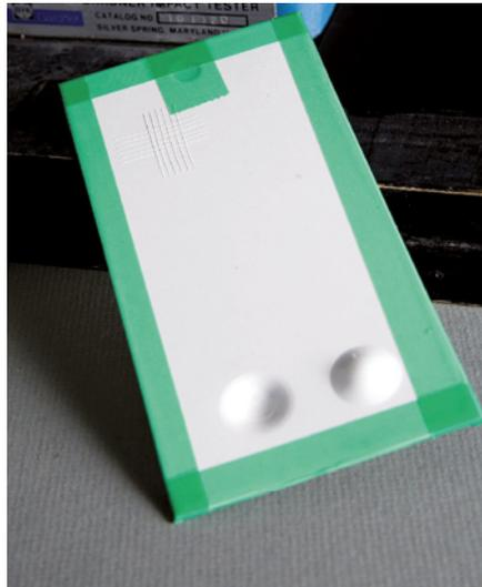
Extensive testing for durability and flexibility shows no resulting cracks, breaks or deterioration of the paint or metal surfaces on panels pre-treated with Dynasylan® HYDROSIL and SIVO® SOL Technology.
