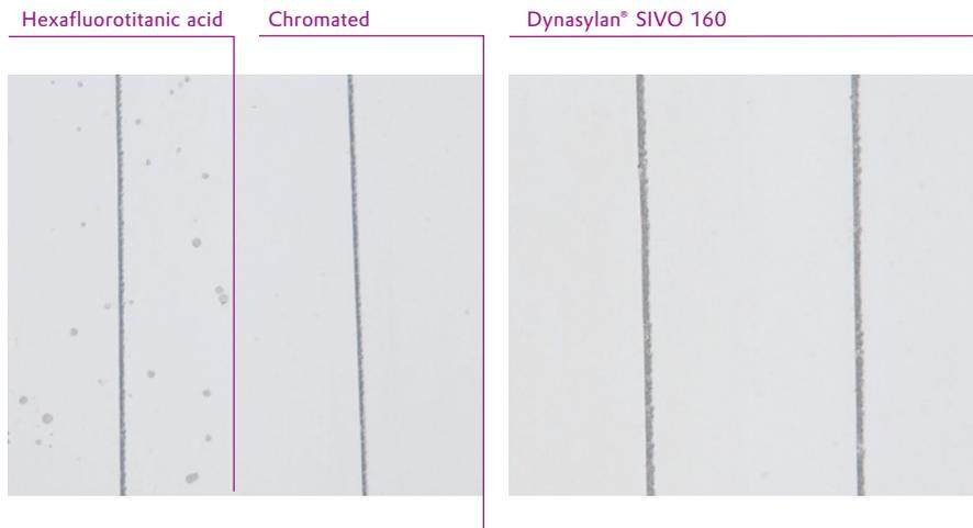
500 hours of acetic acid salt spray testing.
