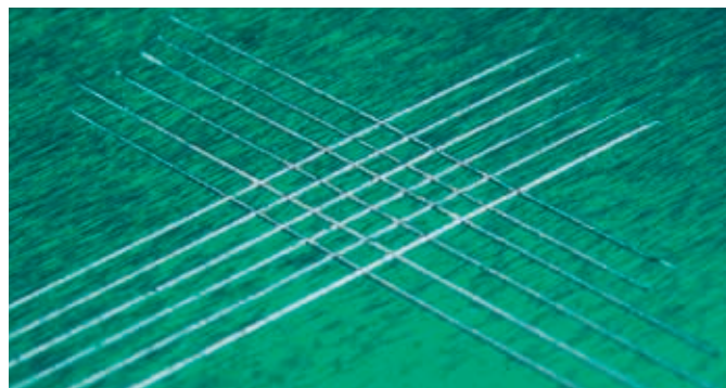
Aluminum substrate pretreated with Dynasylan® HYDROSIL 2909 – Primer
