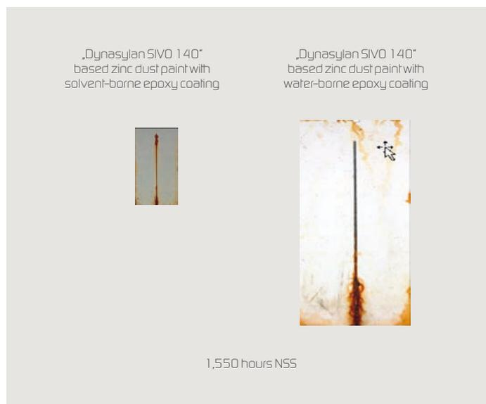
can be overcoated even after two hours. Test panels were coated with a water-borne formulation, cured for two hours at 20 °C and overcoated with an epoxy coating. No adverse effects have so far been found in the performance of these test panels.
