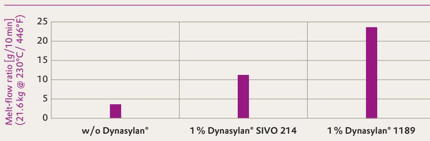
Melt-Flow Ratio (MFR) is increased by a factor of at least four through use of silanes.
