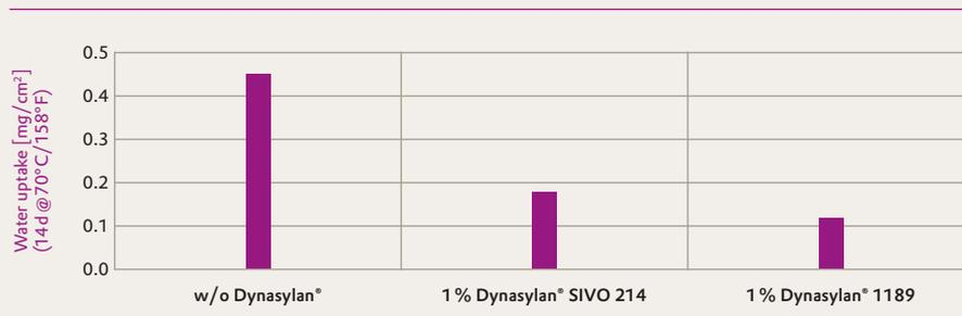
Water uptake is reduced by a factor of four through use of silanes.
