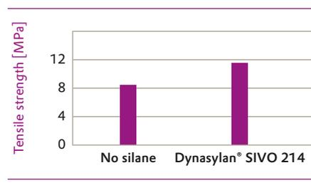
The mechanical properties of magnesium hydroxide-filled polypropylene (PP) compound, with additional maleic anhydride as a coupling agent.
