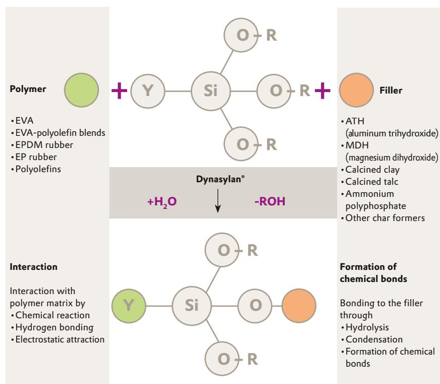
The organofunctional Y-group of the silane links with the polymer. This group must be chosen to ensure maximum compatibility with the resin. A first possibility is to choose a silane that is compatible with the polymer. This ensures improved dispersion. For improved mechanical properties, a reaction needs to take place between the Y-group of the silane and the polymer.
