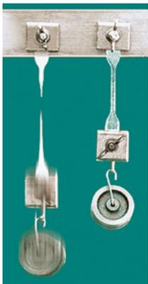
Non-crosslinked polyethylene is very easily deformed as shown in the picture. Through silane crosslinking, the melted polymer retains its dimensional stability and the deformation of the crosslinked polyethylene is minimal (see right part of the picture). By contrast, non-crosslinked polyethylene breaks when exposed to such elevated temperatures (see left part of the picture).
