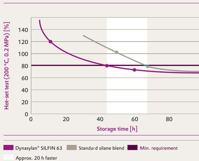
Dynasytan® SILFIN 63 achieves minimum requirement for hot-set test significantly faster.
