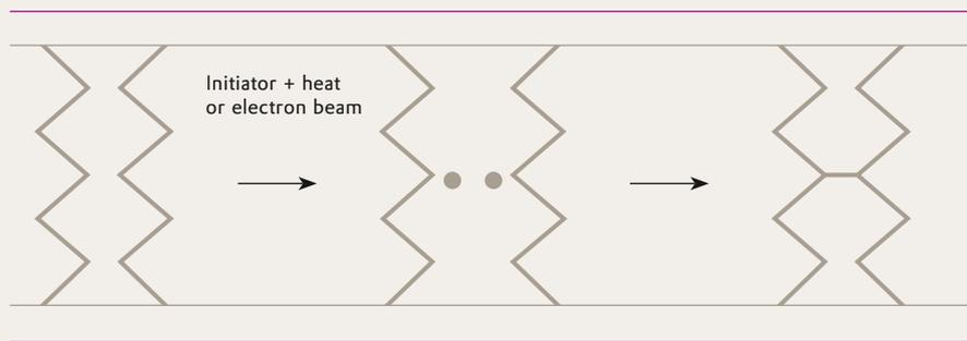
Polyethylene crosslinking through polyethylene radicals.
