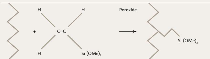
Vinylsilane is attached to the polymer backbone through peroxide grafting.
