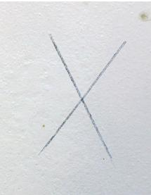
Steel panel with SIVO° SOL Technology <  $1\,\mu$  Film thick thickness. Powder coating cured at 200°C, 10 minutes.
