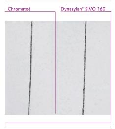
240 hours copper accelerated salt spray test.
