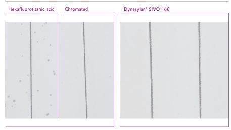
500 hours of acetic acid salt spray testing.
