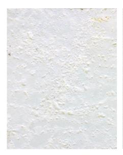
Steel panel with a standard organic primer (5  $\mu).$  Powder coating cured at 200 °C, 10 minutes.
