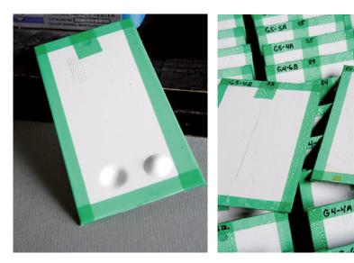
Extensive testing for durability and flexibility shows no resulting cracks, breaks or deterioration of the paint or metal surfaces on panels pre-treated with Dynasylan<sup>®</sup> HYDROSIL and SIVO<sup>®</sup> SOL Technology.
