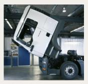
Especially, where high adhesion is required quickly, adhesives formulated on the basis of special silanes have proved to be effective. For example, in heavy goods vehicle production, after only a few minutes, an approx. 40-kg windshield has such a high level of adhesion to the lacquered chassis surface, that the driver's cab could be swung round without any risk at all. Long curing periods are unnecessary so that the vehicles can be moved without restriction and be delivered just in time.
