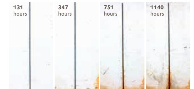
A high zinc content formulation (Table 2) based on Dynasylan® SIVO 140 was applied on shot blasted steel (surface roughness ELK 0.12 – 0.25 mm). Dry film thickness: ~ 70 µm. The zinc-dust paint was overcoated with a water-borne epoxy coating (70 – 80 µm dry film thickness) and placed in a chamber with neutral salt spray fog.
