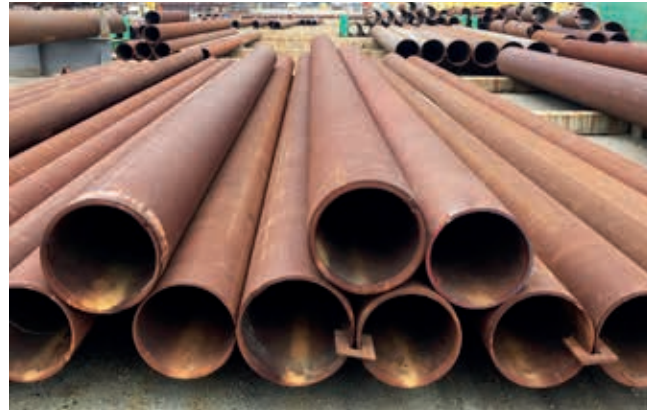
The rust, oil and dirt is removed via shot blasting followed by spray application of the corrosion protection paint.
