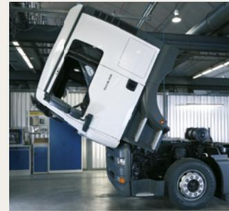
Especially, where high adhesion is required quickly, adhesives formulated on the basis of special silanes have proved to be effective. For example, in heavy goods vehicle production, after only a few minutes, an approx. 40-kg windshield has such a high level of adhesion to the lacquered chassis surface, that the driver’s cab could be swung round without any risk at all. Long curing periods are unnecessary so that the vehicles can be moved without restriction and be delivered just in time.
