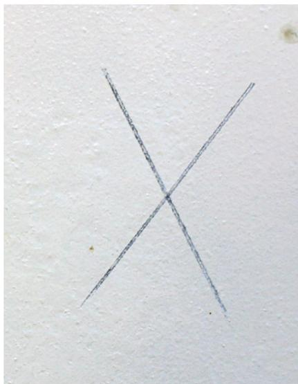
Steel panel with SIVO® SOL Technology < 1 μm Film thickness. Powder coating cured at 200 °C, 10 minutes.
